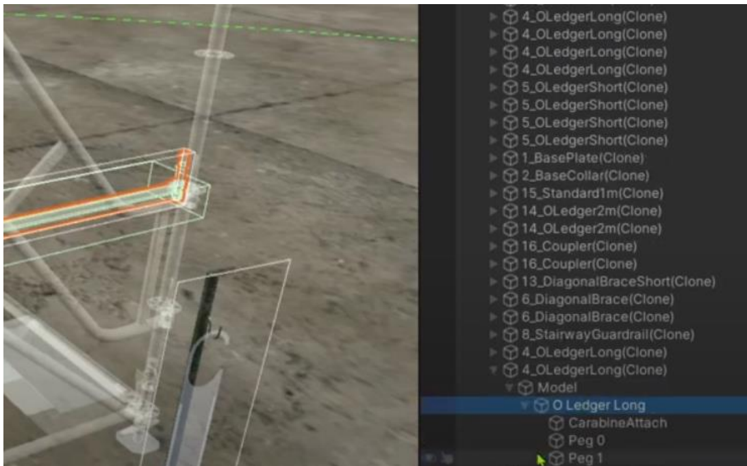
Image 7, Scaffold blueprint objects with pin-functionality
